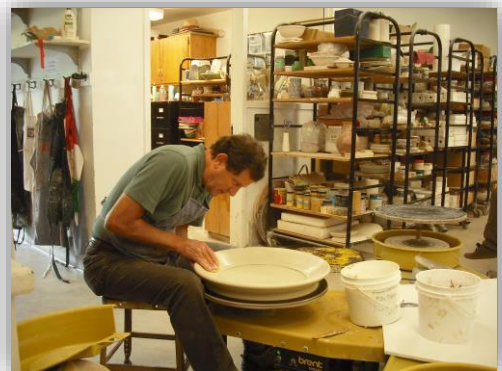
Throwing the ring to form a plate
