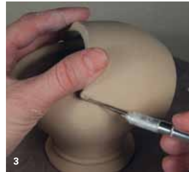
3 Mark the attachment point for the dome, then score, apply slip, and attach the two.
