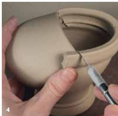
4 Cut a section from a short thrown ring to create the rim of each cruet, place it on the body, cut it to size, and attach.
